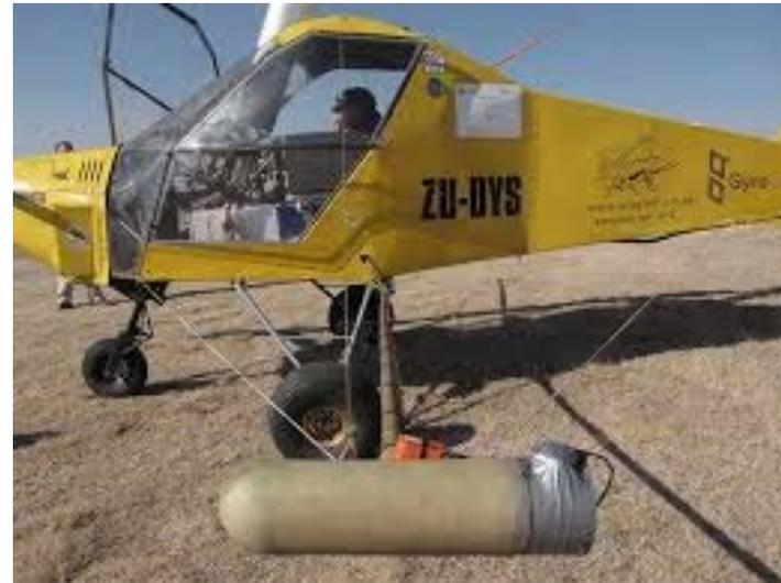
GyroLAG will accommodate up to 7 distinct remote sensing technologies including a range of digital cameras covering the entire IR to UV spectrum, lightweight magnetic, radiometric and gravity sensors.
